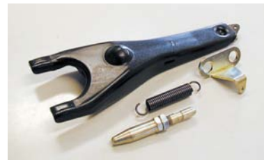
Adjustable fork kit Via return spring, forcibly returns the release fork to position and the adjustable bush rod allows to set the position.
